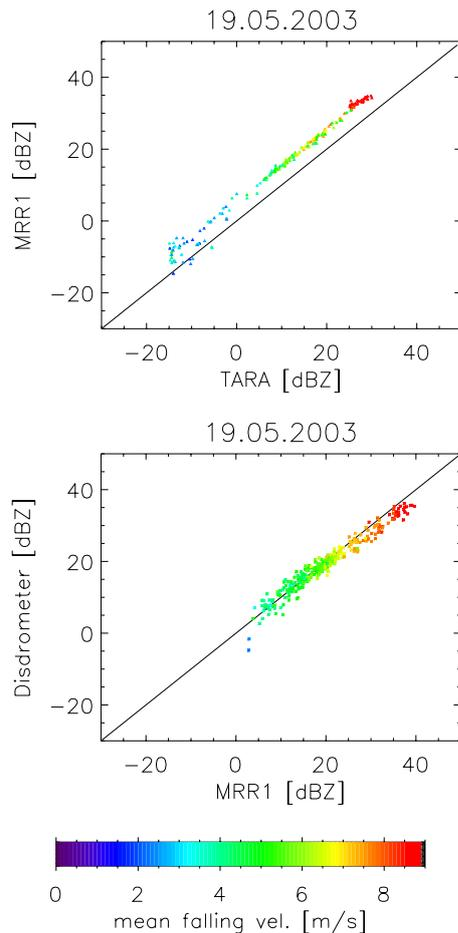
**Fig. 5.** MRR 1 reflectivity values compared to those measured by TARA and calculated from disdrometer spectra for May 19th. The bias between MRR and TARA is believed to be a combination of overestimation by the MRR and underestimation by TARA at low ranges caused by imperfect FMCW transfer functions and possibly insufficient beam overlapping of TARA’s receiver and transmitter. The color coding shows the mean fall velocity measured by the MRR.
