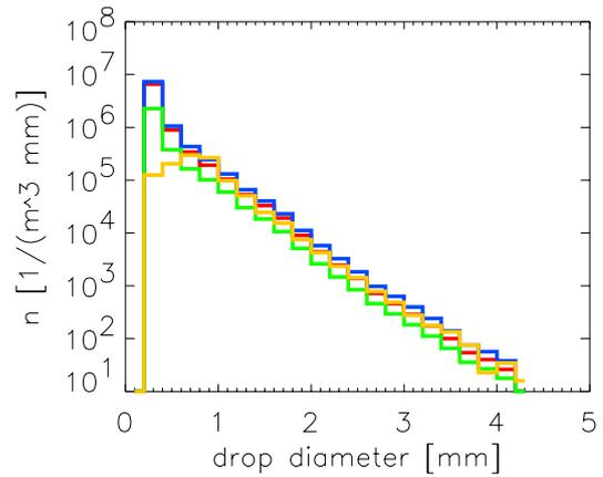
**Fig. 2.** Total drop numbers per cubic meter and diameter interval for a period of 5 days in 22 drop size classes with 0.2 mm interval. Measurements of MRR 1 (height 70 m) are shown in red, MRR 2 in blue, MRR 3 in green, the 2D-Video-Disdrometer in yellow.
