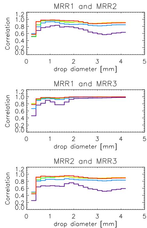
**Fig. 8.** Correlation of drop numbers in 22 drops size classes between the lowest MRR height bin at different integration periods. black: 1 min, blue: 5 min, green: 15 min, yellow: 30 min, red: 1 h. The stronger deviations in larger drops exhibited by MRR 2 against the other MRRs and the disdrometer result from the larger geographic distance.
